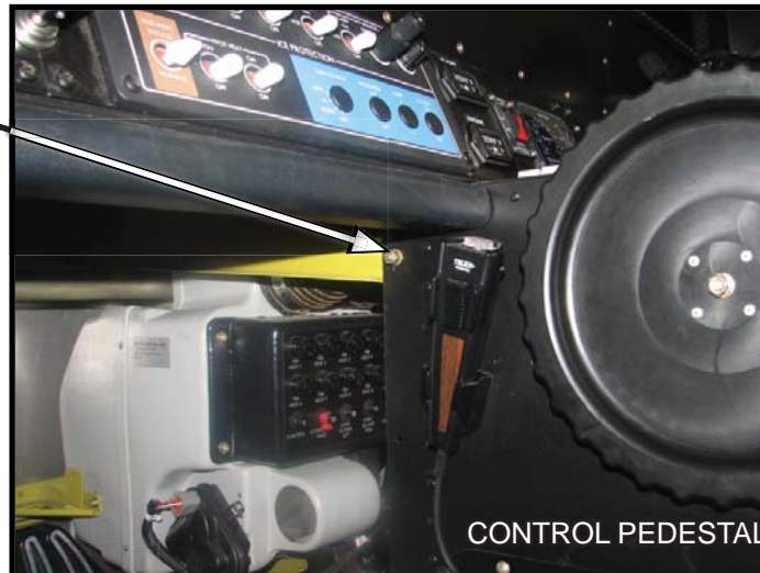
FIGURE 1 : Bolt Inspection Location (Pilot's Side)
