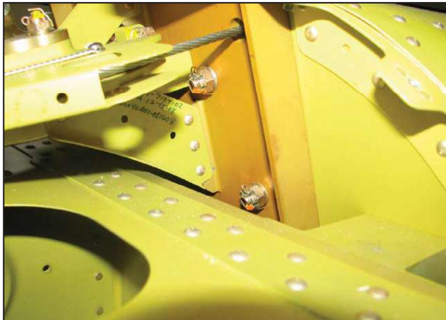
Figure 2 - Outside View of Aftmost Bolts with Tail Cone Removed
