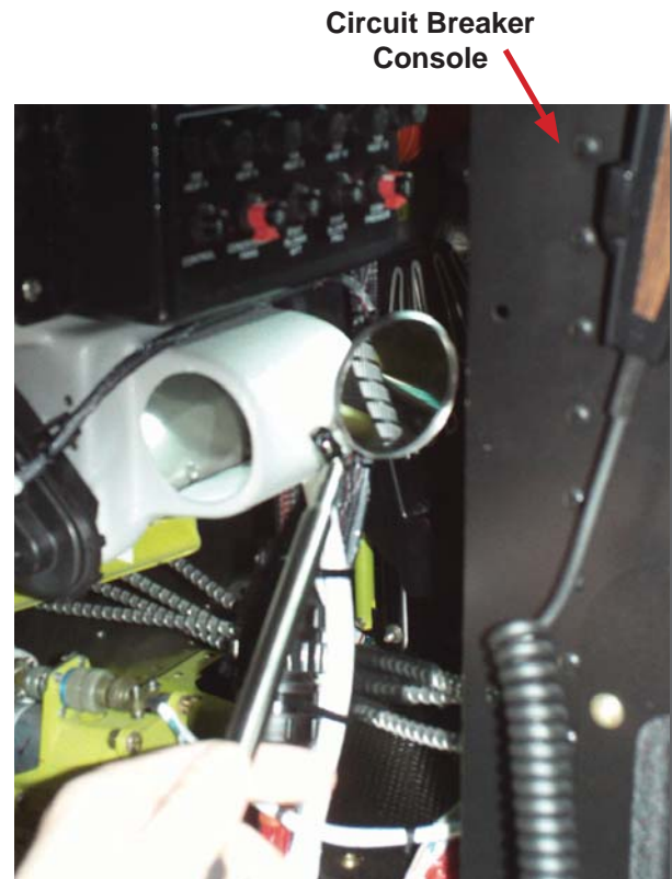
Figure 1-2: Finding the Fuse Sighting Holes
