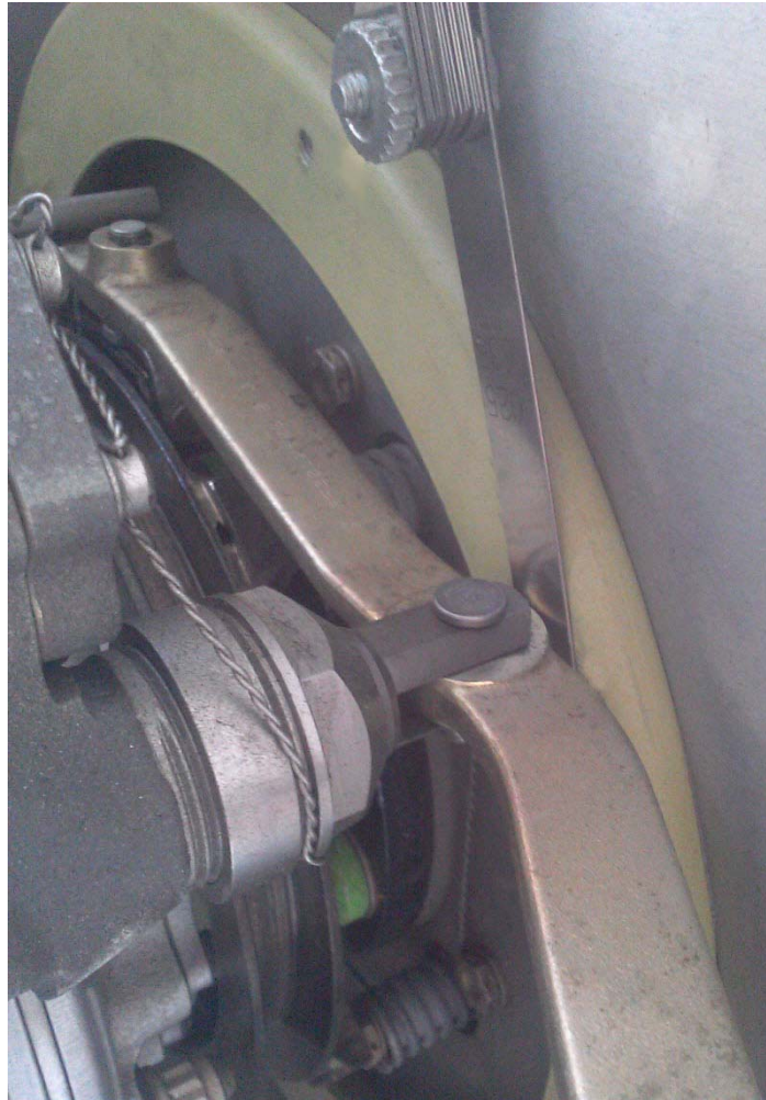
Figure 5-9: Measure Beta Arm/Slinger Ring Gap
