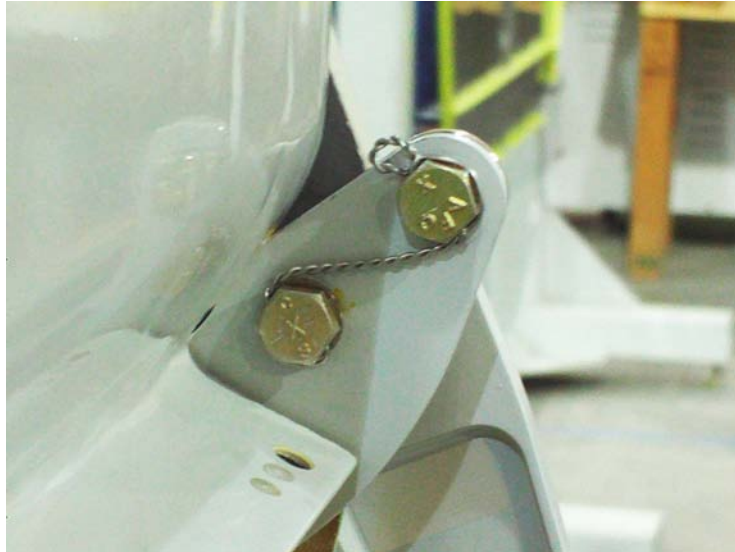
Figure 5-3: Safety Wire Installation
